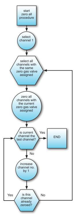
Fig. 7-4: Zero All Calibration Procedure Flow Chart
